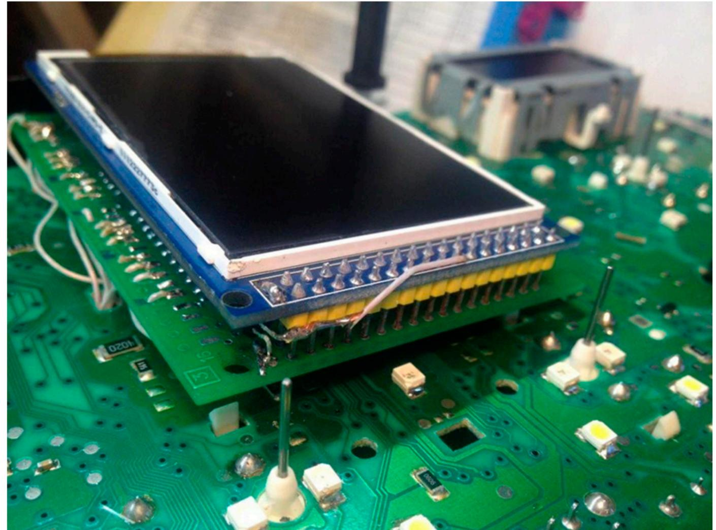
**3.4. For greater reliability, when the module is already installed on the board, and you calibrated it in the window so that there were no distortions, it is better to fix it. Its hot glue along the edges of the module.**
