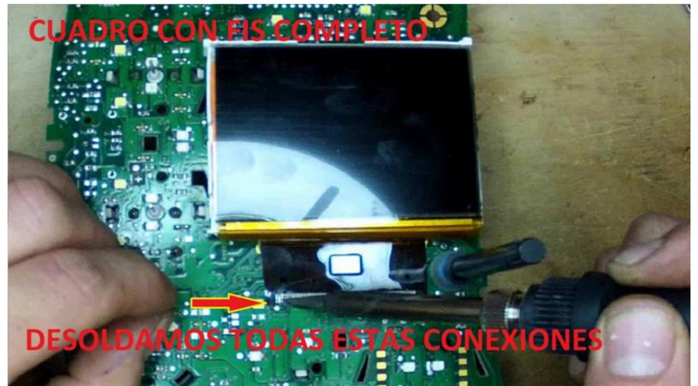
**1.5.2. On some instrument panels, the plastic base of the OEM FIS is soldered to the board pretty hard, to dismantle it — remove the tin, using a soldering iron and a special vacuum.**
