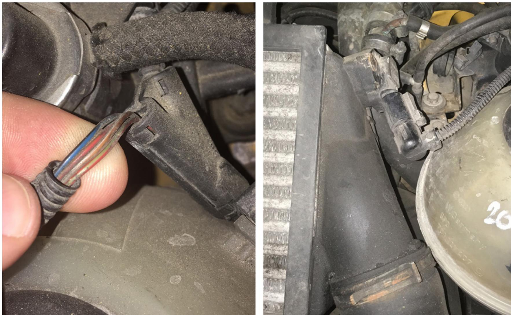
**11.3. Usually it is blue - gray wire (blue with a gray bar) to the incoming on the 101st contact of a smaller brain connector. (for a gasoline engine)**
