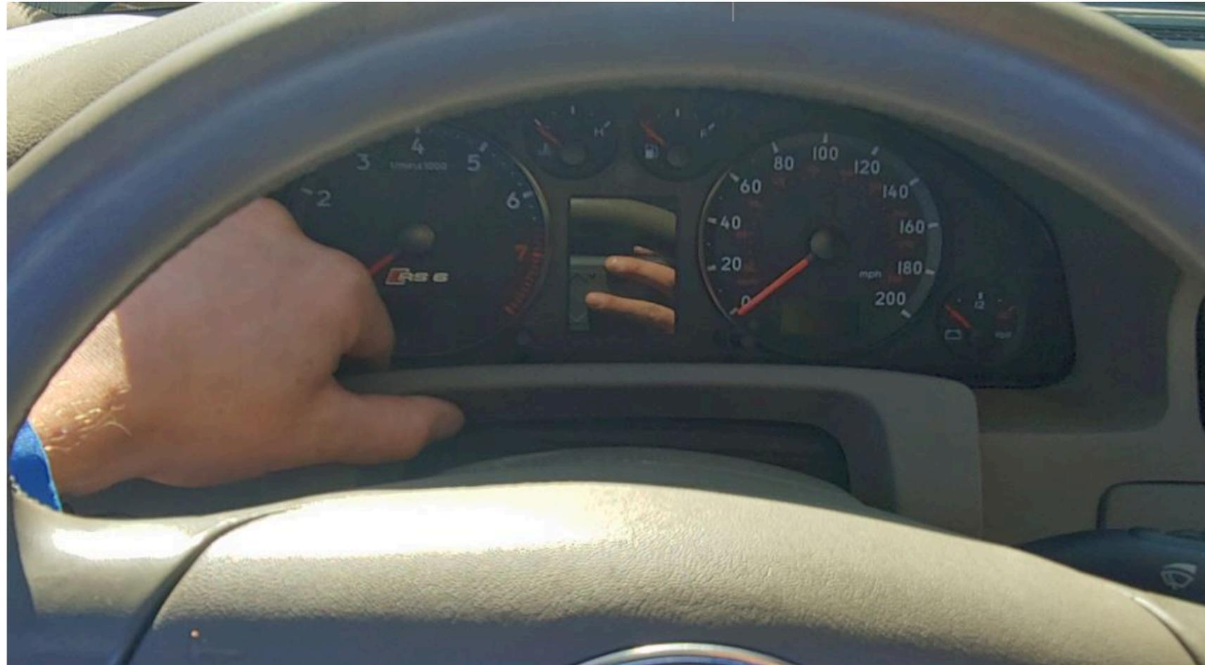
2) (audi b5 has 2 torx 20 bit screws) (audi c5 !!!GLUED PHILLIPS!!! MAKE SURE TO HAVE A TIGHT FITTING PHILLIPS WITH HEAVY PRESSURE)
